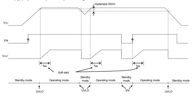
Fig.22 Soft start, Shutdown, UVLO timing chart
