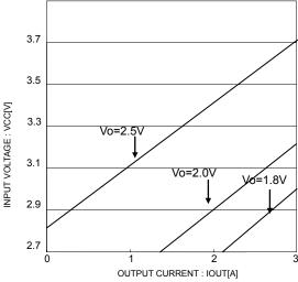
Fig.35 minimum input voltage in each output voltage
