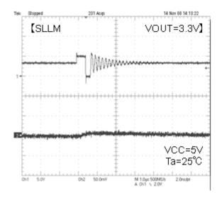
Fig.15 SW waveform Io=10mA
