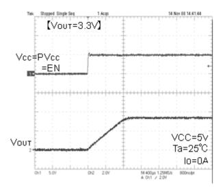
Fig.14 Soft start waveform
