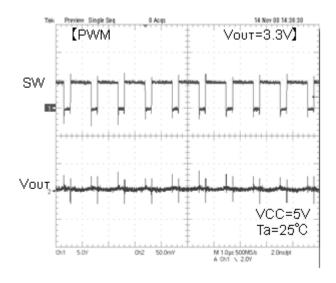
Fig.16 SW waveform Io=3A
