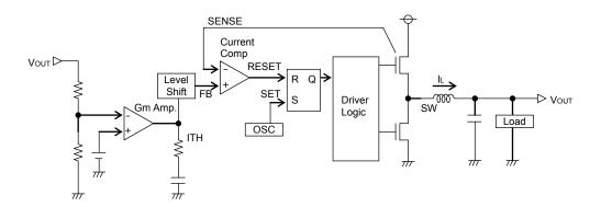
Fig.19 Diagram of current mode PWM control
