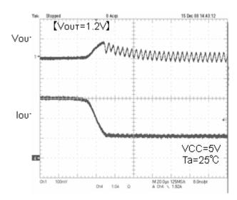
Fig.18 Transient Response Io=3→1A(10µs)
