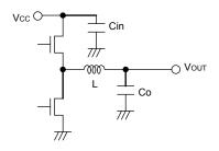
Fig.30 Input capacitor
