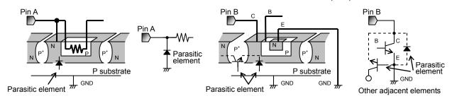
Fig.38 Simplified structure of monorisic IC
