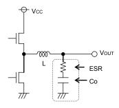
Fig.29 Output capacitor
