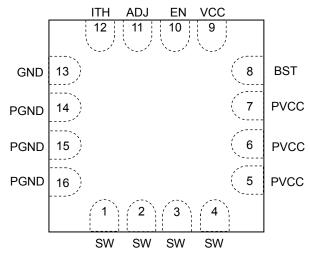
Fig. 2 Pin Configuration
