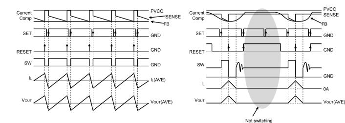
Fig.20 PWM switching timing chart
