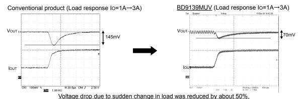
Fig.24 Comparison of transient response
