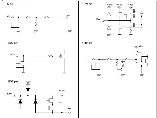
Fig.37 I/O equivalence circuit
