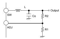
Fig.34 Determination of output voltage
