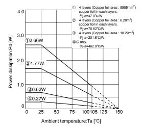
Fig.27 Thermal derating curve (VQFN016V3030)
