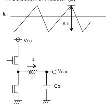
Fig.28 Output ripple current
