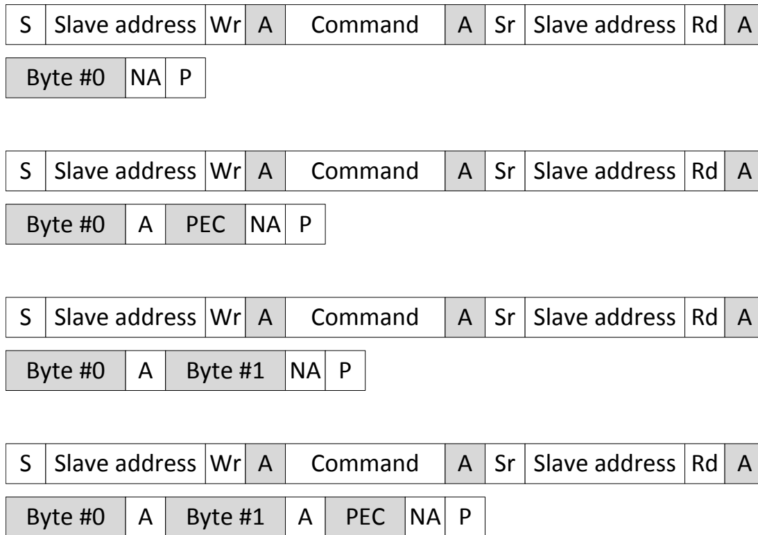
Figure 26-6. Read Byte and Read Word Messages with and without PEC
