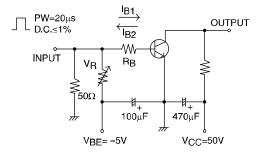
$I_{C}=10I_{B1}=-10I_{B2}=2A$ For PNP, the polarity is reversed.
