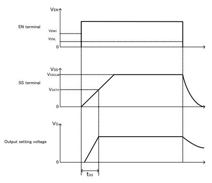
Fig.12 ON/OFF transition wave form in EN controlling
