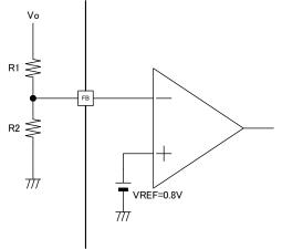
Fig.16 Output voltage setting circuit
