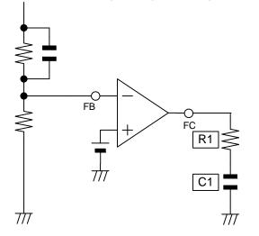
Fig.19 Phase amends part external circuit chart
