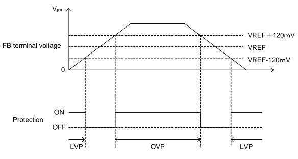
Fig.14 Output voltage error detection range
