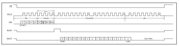
FIGURE 8. External Clock Mode 32 Clocks Per Conversion.
