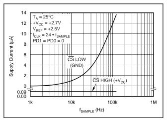
FIGURE 11. Supply Current vs State of CS.
