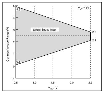
FIGURE 3. Single-Ended Input—Common Voltage Range vs V<sub>REF</sub>.
