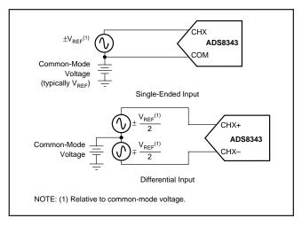
FIGURE 2. Methods of Driving the ADS8343—Single-Ended or Differential.
