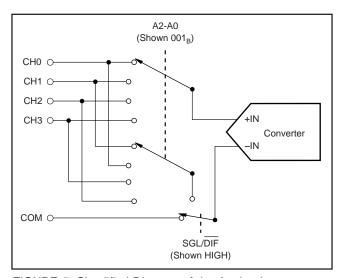
FIGURE 5. Simplified Diagram of the Analog Input.
