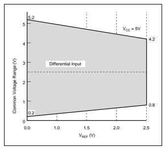
FIGURE 4. Differential Input—Common Voltage Range vs V<sub>REF.</sub>
