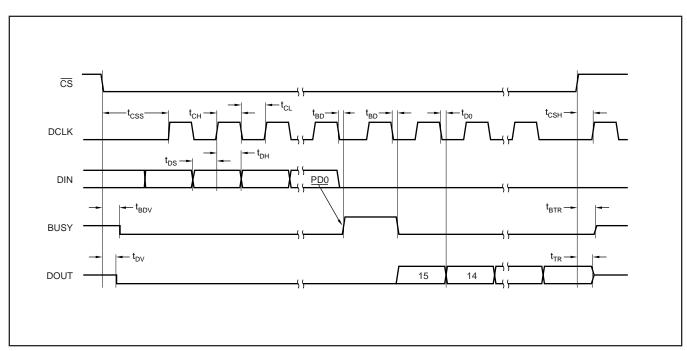
FIGURE 7. Detailed Timing Diagram.
