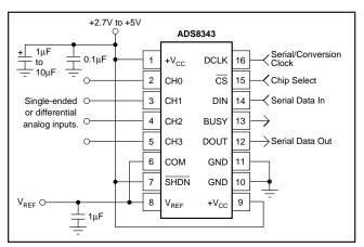
FIGURE 1. Basic Operation of the ADS8343.
