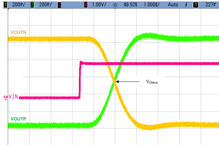
Figure 51. Step Response of the AMC1311B
