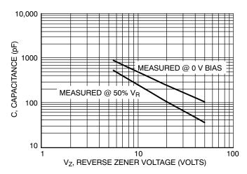
Figure 8. Capacitance versus Reverse Zener Voltage
