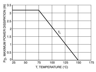
Figure 1. Steady State Power Derating
