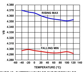
FIGURE 17. BATTERY VOLTAGE OVP THRESHOLDS vs
