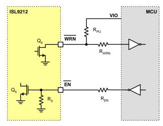
FIGURE 24. DIGITAL SIGNAL INTERFACE BETWEEN ISL9212B AND MCU
