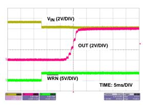
FIGURE 5. TRANSIENT WHEN THE INPUT VOLTAGE STEPS FROM 7.5V TO 6.5V
