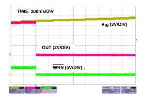
FIGURE 4. CAPTURED WAVEFORMS WHEN THE INPUT GRADUALLY RISES TO THE INPUT OVERVOLTAGE THRESHOLD
