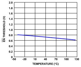
FIGURE 20. EN INPUT THRESHOLD vs TEMPERATURE
