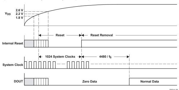
Figure 22. Internal Power-On Reset Timing
