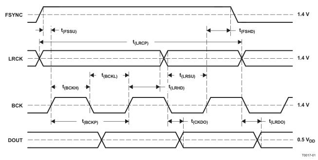
Timing measurement reference level is  $(V_{IH} + V_{IL}) / 2$ . Rise and fall times are measured from 10% to 90% of IN to OUT signal swing. Load capacitance of DOUT is 20 pF.
