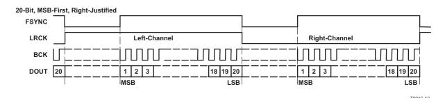
Figure 25. Audio Data Format (Master Mode: FSYNC, LRCK, and BCK Work as Outputs)
