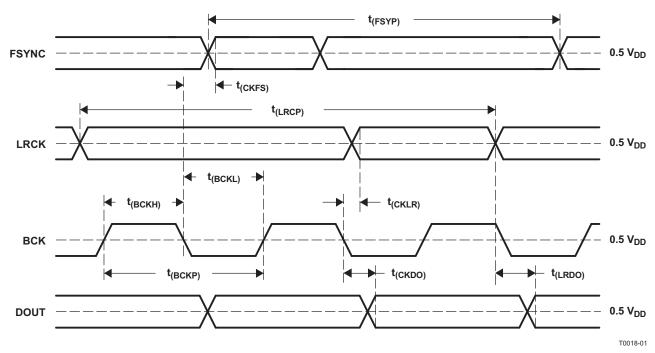
Timing measurement reference level is  $(V_{IH} + V_{IL}) / 2$ . Rise and fall times are measured from 10% to 90% of IN to OUT signal swing. Load capacitance of all signals is 20 pF.
