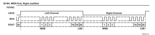
Figure 23. Audio Data Format (Slave Mode: FSYNC, LRCK, and BCK Work as Inputs)
