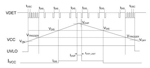
Figure 1. Typical Waveforms of APR3415B
