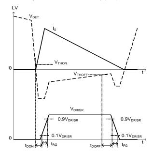
Figure 2. Typical Waveforms of APR3415B
