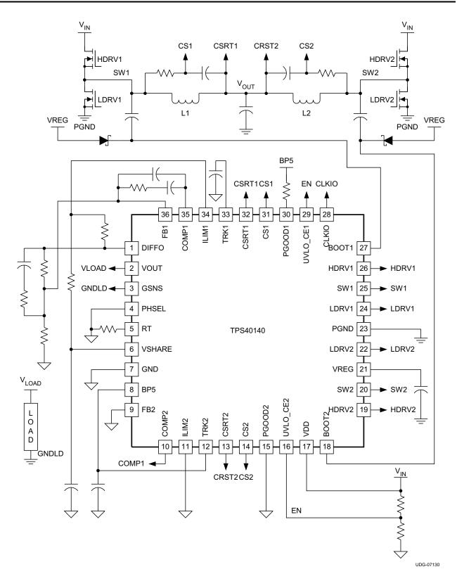
Figure 5-11. Typical Applications Circuit, 2-Phase Mode
