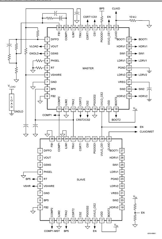
Figure 5-13. Typical Applications Circuit, 4-Phase Mode
