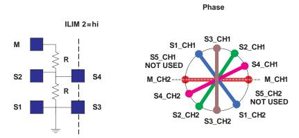
Figure 5-22. Ten-Phase System with Slaves Not Attached
