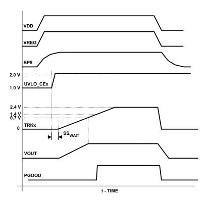
Figure 5-1. Typical Start-Up and Shut-Down Sequence
