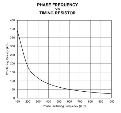
Figure 5-6. Phase Switching Frequency vs Timing Resistance
