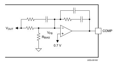
Figure 5-5. Setting the Output Voltage with R<sub>BIAS</sub>
