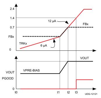
Figure 5-2. Soft-Start with Pre-Biased Output Waveforms
