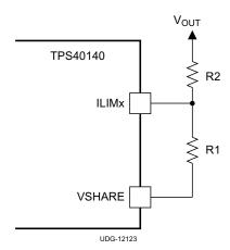
Figure 5-10. Selecting Overcurrent Threshold Resistors, R2 and R1
