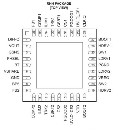
The TPS40140 is a versatile controller that can operate as a single controller or 'stacked' in a multi-controller configuration. A TPS40140 has two channels that may be configured as a multi-phase (single output) or as a dual, with two independent output voltages. The two channels of a single controller always switch 180 degrees out-of-phase. See below for further discussion on the Clock and voltage master and Clock and Voltage slave.
