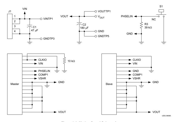
Figure 6-6. Mother Board Schematic
