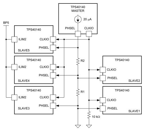
Figure 5-18. Master Controller and Five Slave Controllers, 12-Phases
