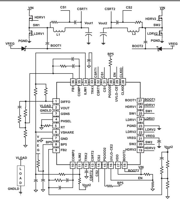
Figure 5-12. Typical Applications Circuit, Dual Mode
