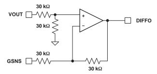
Figure 5-4. Differential Amplifier Configuration
