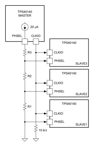
Figure 5-17. Master Controller and Three Slave Controllers, Eight Phases
