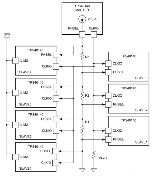
Figure 5-19. Master Controller and Seven Slave Controllers, 16 Phases
