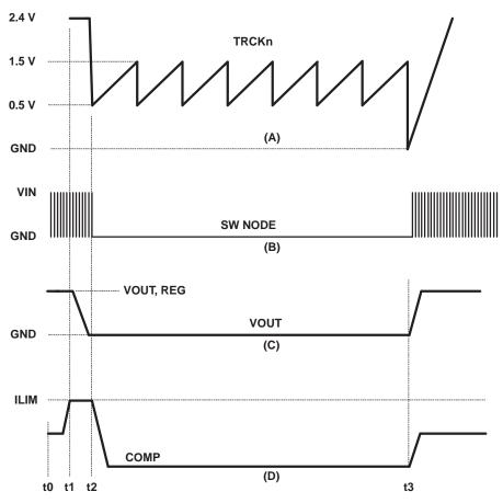
Figure 5-9. Hiccup Mode and Recovery
