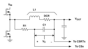
Figure 5-23. Inductor DCR Current Sense Approach
