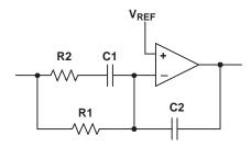
Figure 6-1. Type II Compensator
