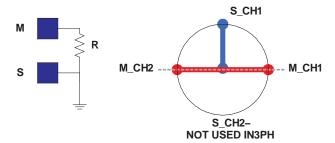
Figure 5-21. Phase System: 2 Channels of the Master and 1 Channel of the Slave
