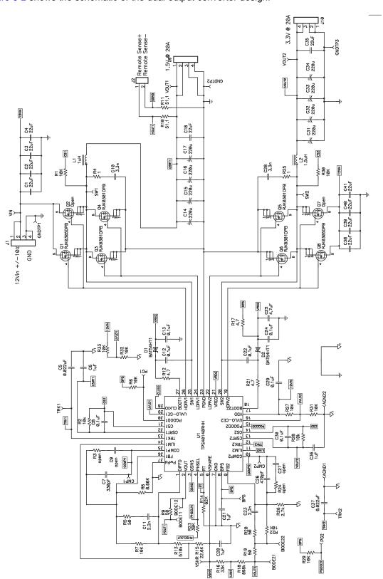
Figure 6-2. Dual-Output Converter Schematic
