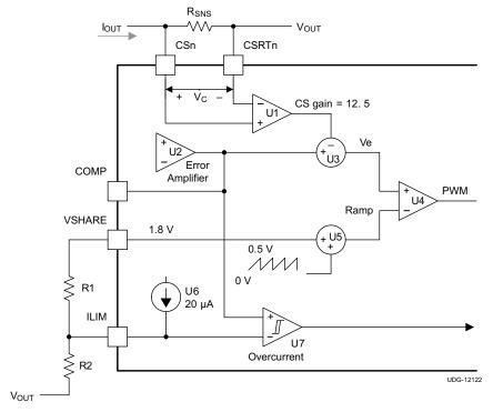
Figure 5-8. Output Current Sensing and Overcurrent Detection
