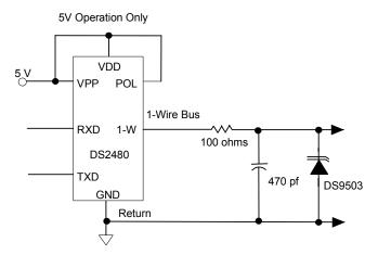
To protect the 1-Wire port of the DS2480B from electrostatic discharge it is recommended to use a low-capacitance ESD protection diode, such as the DS950x devices. For 5V operation a single device is sufficient. For EPROM programming two DS950x devices must be connected in series to achieve a high enough breakdown voltage.
