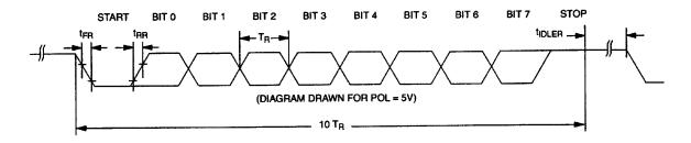
Figure 13. RECEIVE DELAY TIMING
