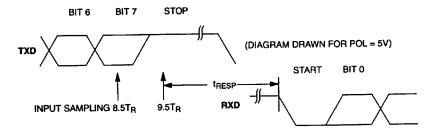
Figure 14. RS232 DATA TIMING TXD LINE
