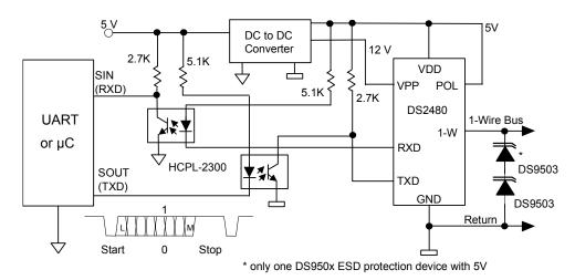
The circuit in Figure 11d is essentially the same as in Figure 11a. The main difference is the opto-isolation. The characteristics of the opto-isolators are not very critical. Using a different type will affect the values of the resistors that limit the current through the LEDs and bias the photo transistors.
