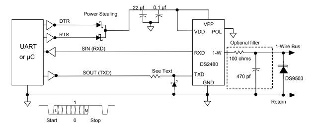
The signals DTR and RTS provide the power to operate the DS2480B. The resistor in the TXD line and the Schottky diode limit the negative voltage at the TXD pin of the DS2480B to 0.3V maximum. The resistor is typically  $4.7k\Omega$ . If the inverting driver is current-limited to 1mA the resistor is not required.
