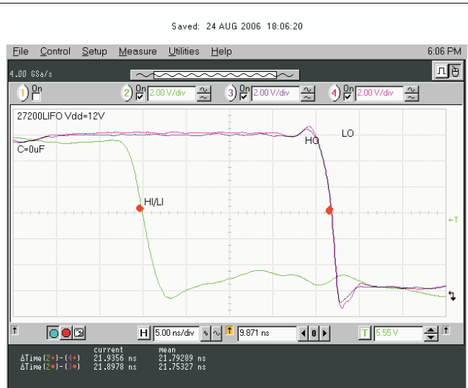
Figure 31. V_{LO} and V_{HO} Falling Edge Delay Matching
