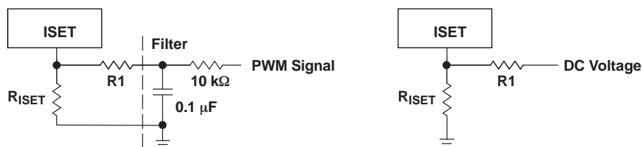
Figure 14. Analog Dimming Uses an External Voltage Source to Control the Output Current
