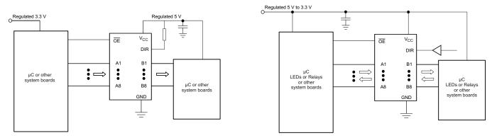
Figure 5. Typical Application Diagram
