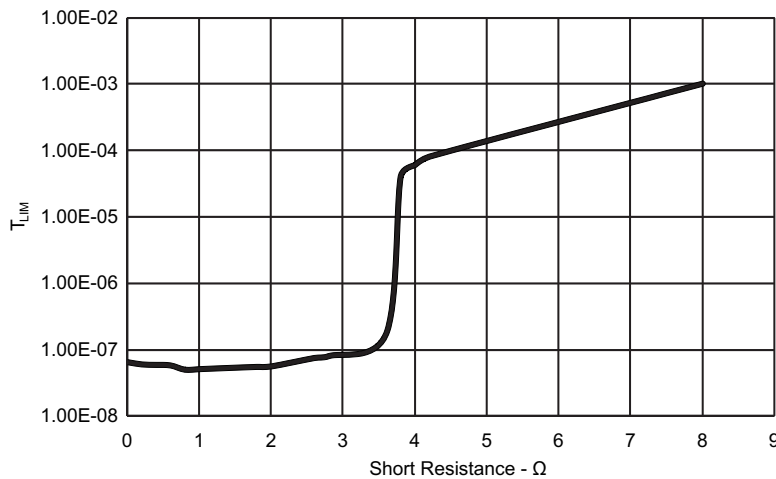
Figure 11. Overcurrent Response Time vs Short Resistance
