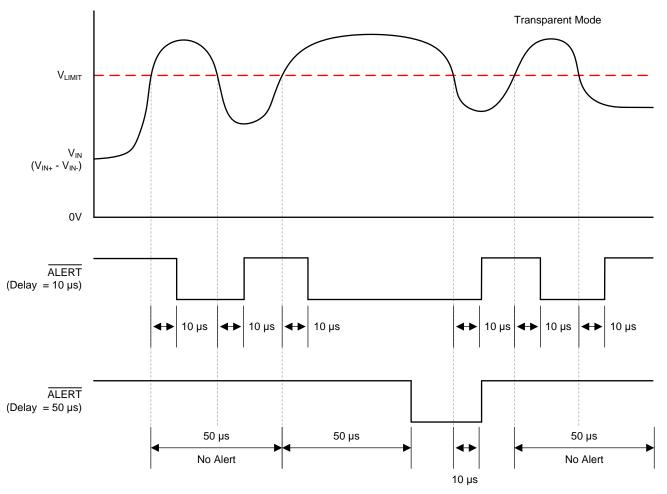
Figure 22. DELAY Terminal Settings
