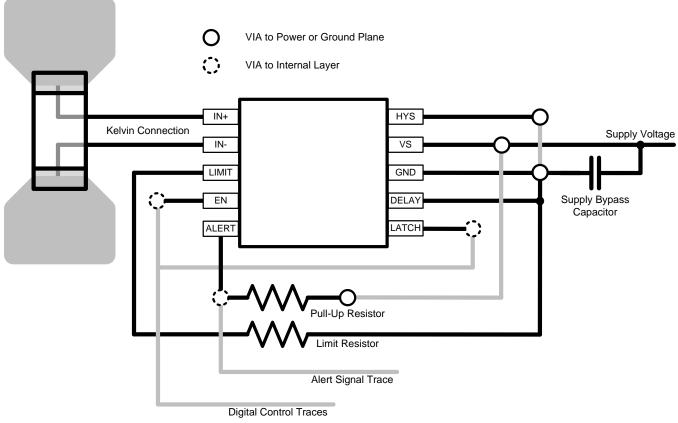
NOTE: Connect the limit resistor directly to the GND terminal.
