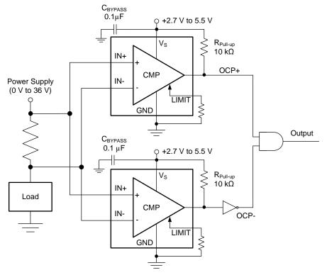
Figure 37. Window Comparator Application
