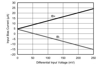
Figure 31. Input Bias Current vs Differential Input Voltage
