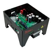
The InstaSPIN-FOC<sup>TM</sup> and InstaSPIN-MOTION<sup>TM</sup> technologybased high-voltage motor control kit provides an easy way to evaluate the Piccolo microcontroller and TI analog in a
