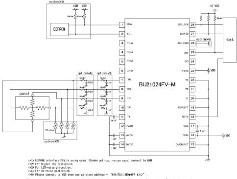
Example 4: BU21024FV-M Application Circuit (2-wire Serial bus)
