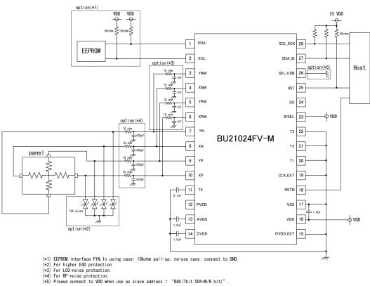
Example 6: BU21024FV-M Application Circuit (2-wire Serial bus, using monitor terminals)
