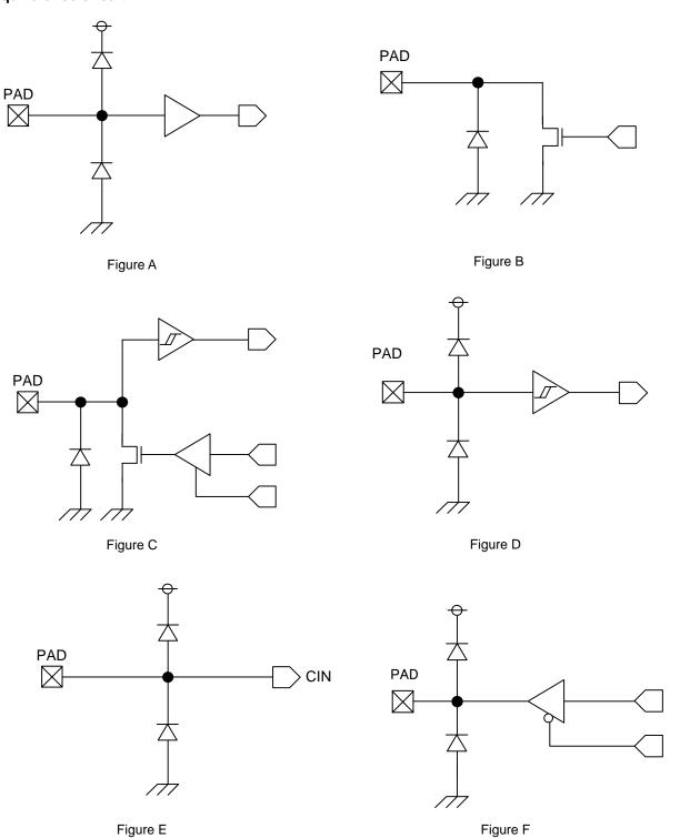
Figure I/O Equivalent Circuit
