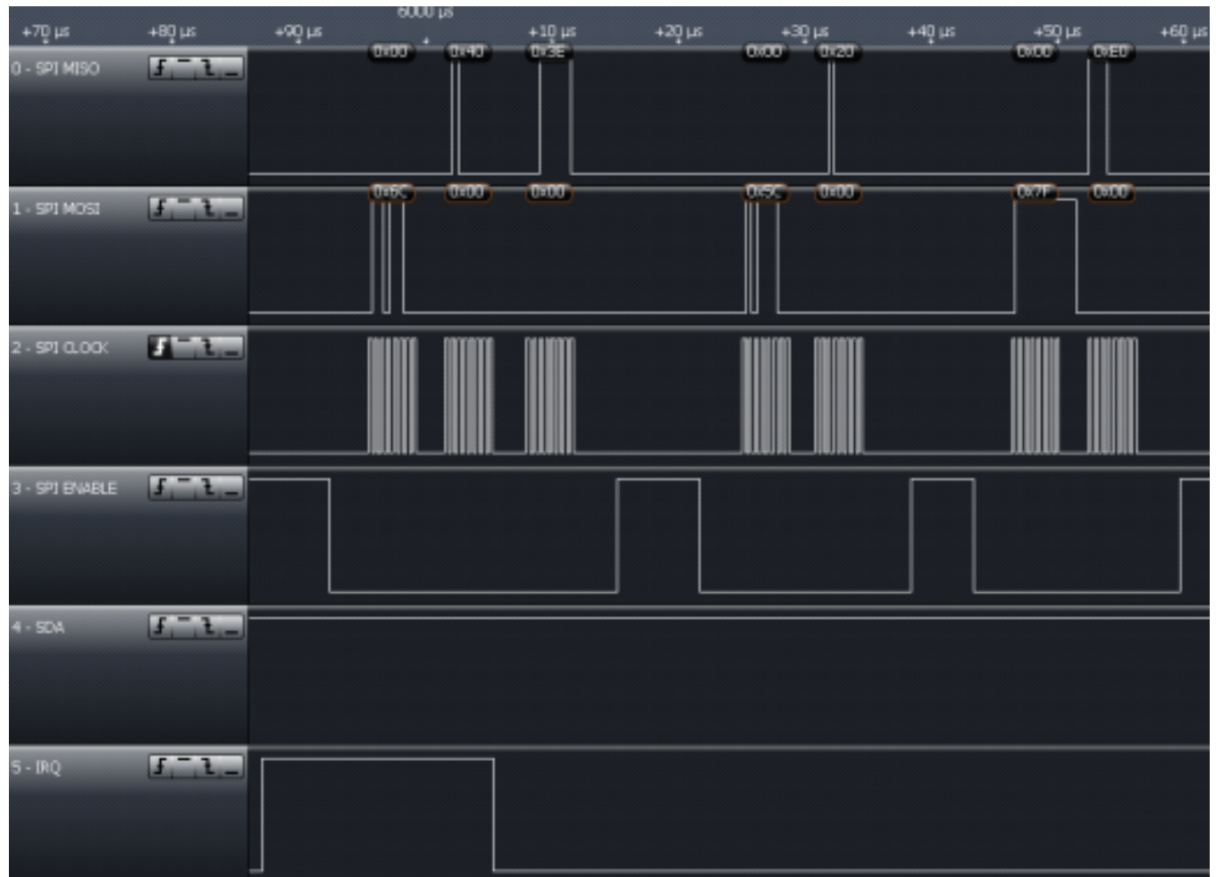
Figure 5-24. Second IRQ After Inventory Command
