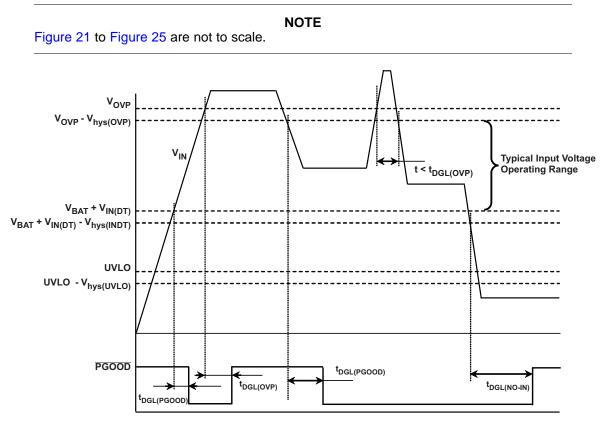
Figure 21. Power-Up, Power-Down, Power Good Indication
