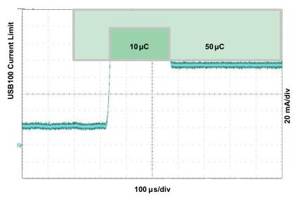
Figure 14. USB-IF Inrush Current Test
