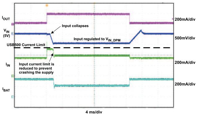
Figure 15. V<sub>IN</sub>-DPM Waveform
