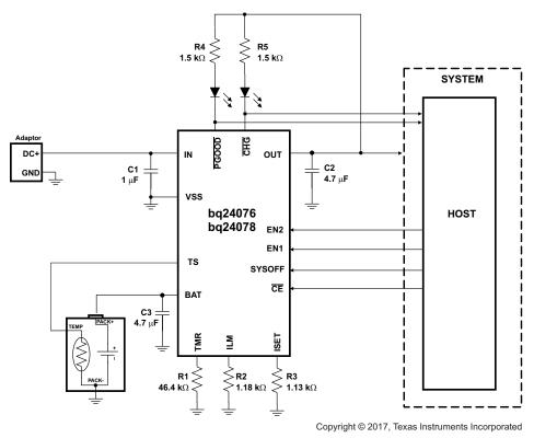
Figure 26. Using bq24076/bq24078 in a Host-Controlled Charger Application
