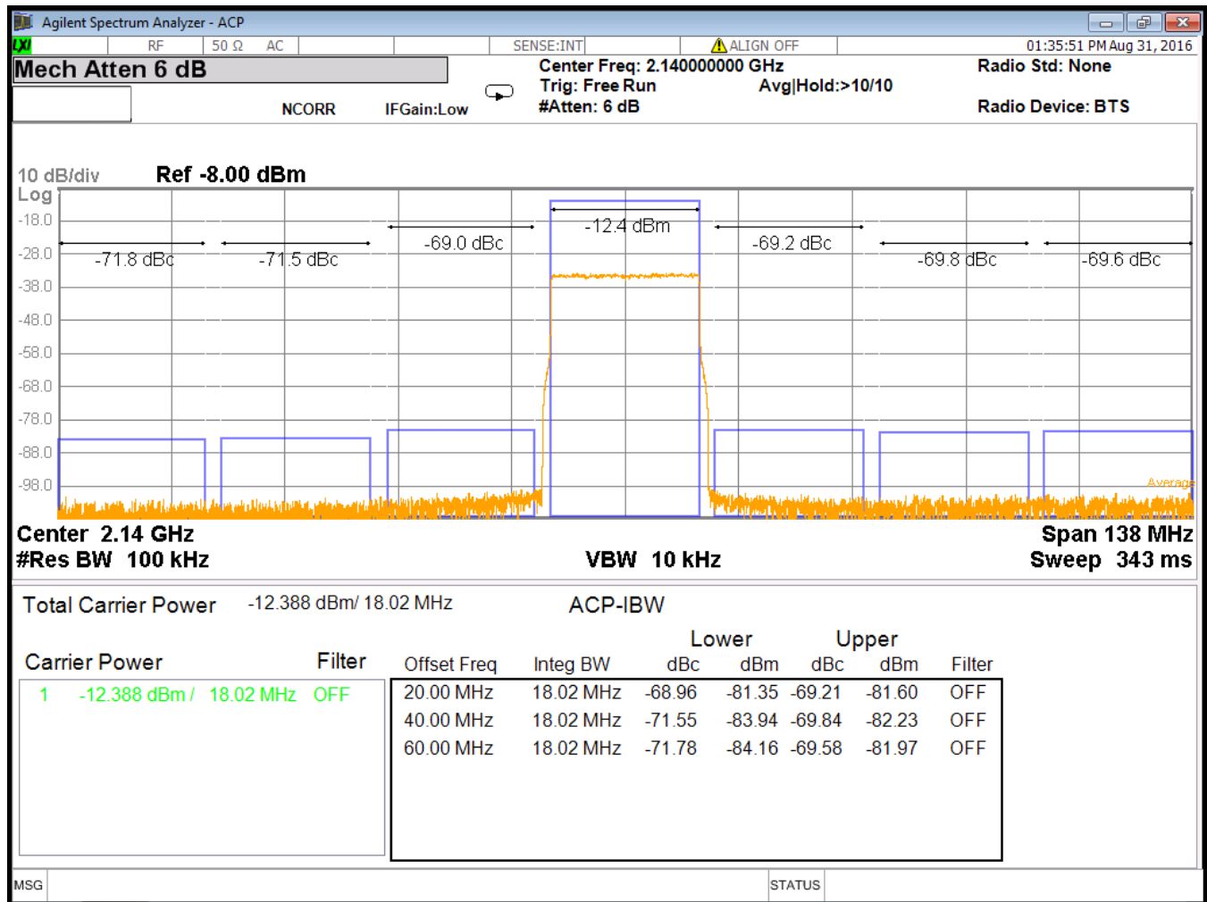
Figure 169. Dual band ACPR Performance in Downlink Band 1 with On-chip PLL
