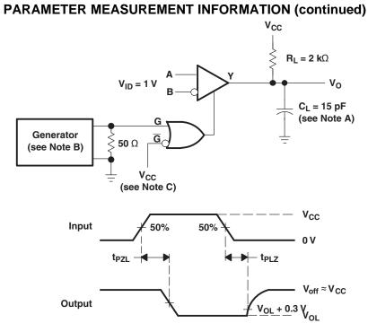
Figure 3. Test Circuit and Voltage Waveforms,  $t_{PZL}$  and  $t_{PLZ}$
