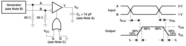
Figure 1. Test Circuit and Voltage Waveforms, tPLH and tPHL
