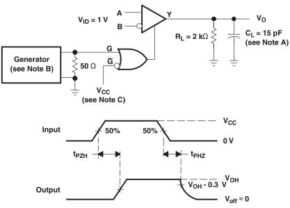
Figure 2. Test Circuit and Voltage Waveforms,  $t_{\text{PZH}}$  and  $t_{\text{PHZ}}$
