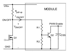
Figure 31. Circuit configuration for using negative logic On/OFF.
