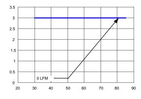
Figure 23. Derating Output Current versus Local Ambient Temperature and Airflow (VIN = 3.3dc, Vo=1.2 Vdc)
