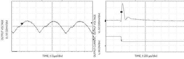
Figure 8. Typical Output Ripple and Noise (VIN = 5.0V dc, Vo = 0.75Vdc, Io=3A).
