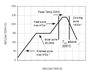
Figure 37. Reflow Profile for Tin/Lead (Sn/Pb) process.
