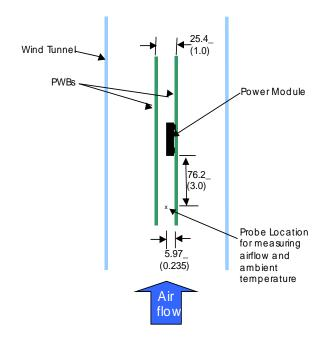
Figure 35. Thermal Test Set-up.
