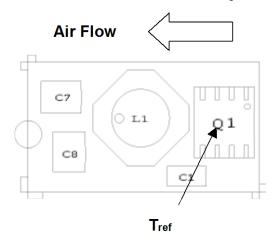
Figure 34. Tref Temperature measurement location.
