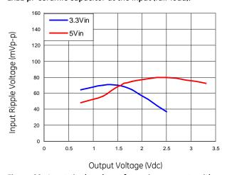
Figure 29. Input ripple voltage for various outputs with 1x47 µF ceramic capacitor at the input (full load).
