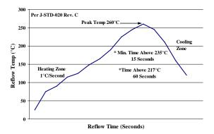
Figure 39. Recommended linear reflow profile using Sn/Ag/Cu solder.
