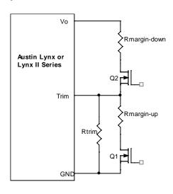
Figure 33. Circuit Configuration for margining Output voltage.
