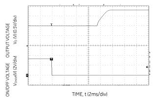
Figure 17 Typical Start-Up Using Remote On/Off with Prebias (VIN = 3.3Vdc, VO = 1.8Vdc, IO = 1.0A, VD = 1.0Vdc).
