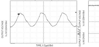
Figure 9. Typical Output Ripple and Noise (VIN = 5.0V dc, Vo = 3.3Vdc, Io=3A).
