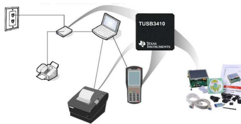
Figure 6-1. Typical Example for TUSB3410 as USB to UART Bridge
