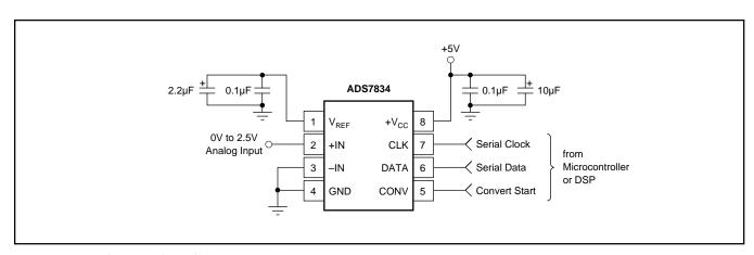
FIGURE 1. Basic Operation of the ADS7834.
