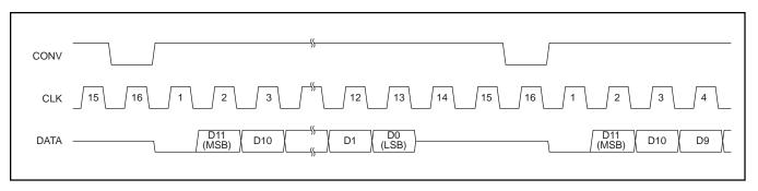
FIGURE 8. Typical DSP Interface Timing.
