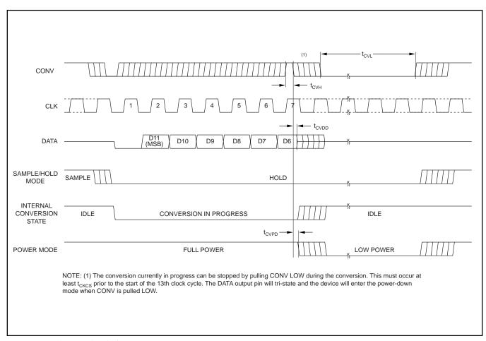
FIGURE 6. Short-cycle Timing.
