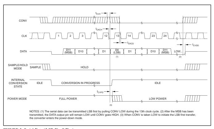
FIGURE 5. Serial Data "LSB-First" Timing.
