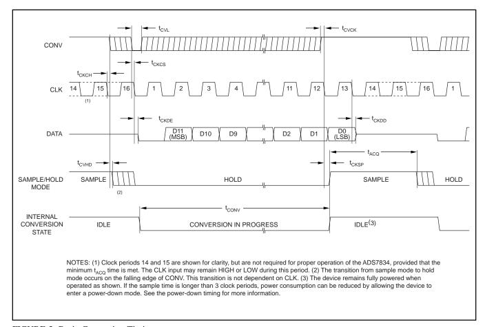
FIGURE 3. Basic Conversion Timing.
