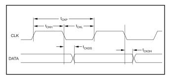
FIGURE 2. Serial Data and Clock Timing.
