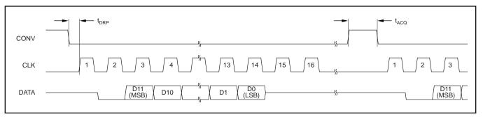
FIGURE 9. Typical SPI/QSPI Interface Timing.
