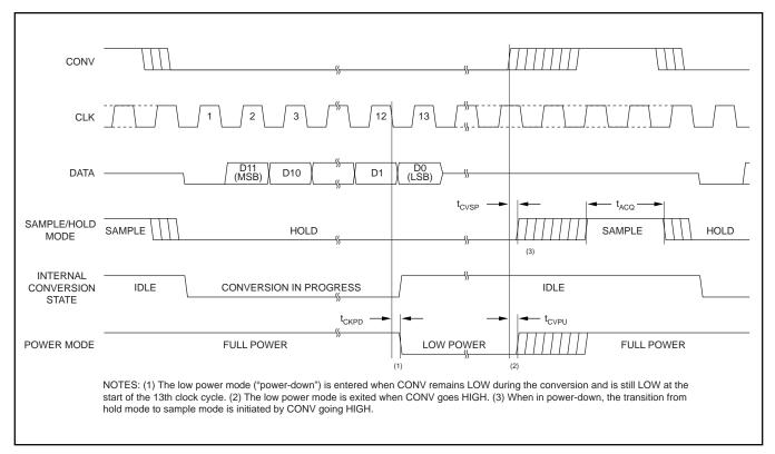
FIGURE 4. Power-down Timing.
