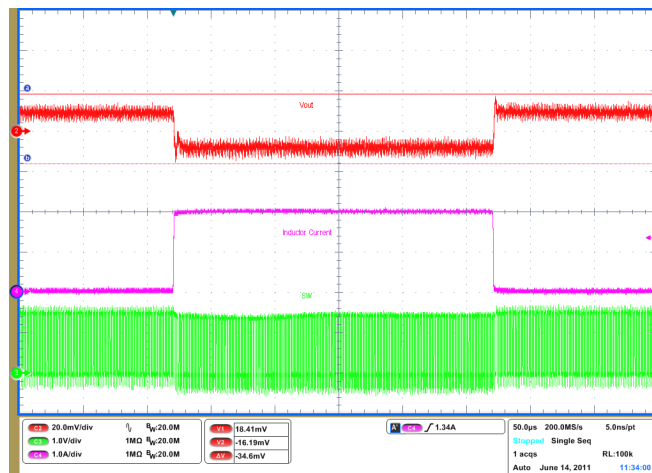
Figure 10. Droop Configuration Transient Response CH 2: V OUT (20 mV/div) CH 4: I LOAD (1 A/div) CH 3: SW (1 V/div)
