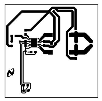
Figure 23. Recommended SD PCB Layout Top Layer
