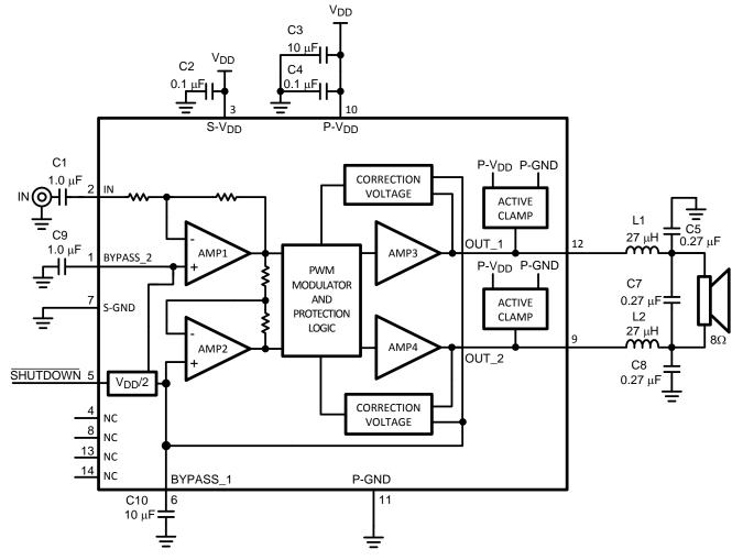
Figure 2. Typical Audio Amplifier Application Circuit
