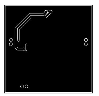
Figure 24. Recommended SD PCB Layout Bottom Layer
