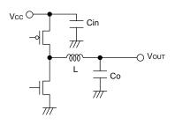
Fig.29 Input capacitor
