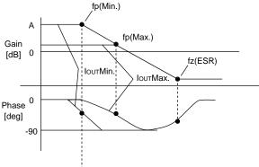
Fig.30 Open loop gain characteristics
