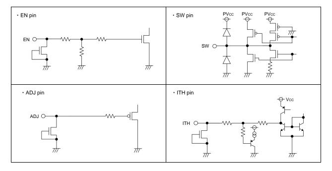
Fig.36 I/O equivalence circuit
