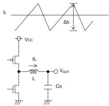
Fig.27 Output ripple current
