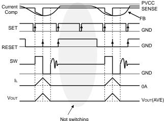
Fig.23 SLLM<sup>TM</sup> switching timing chart
