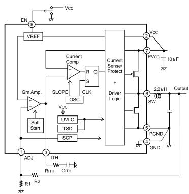
Fig.2 BD9130EFJ Block Diagram
