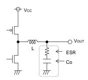
Fig.28 Output capacitor
