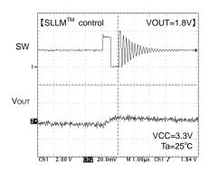
Fig.13 Soft start waveform
