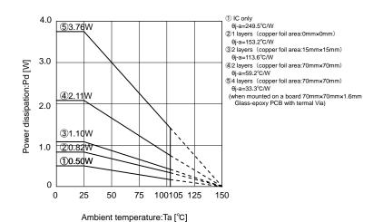
Fig.26 Thermal derating curve (HTSOP-J8)
