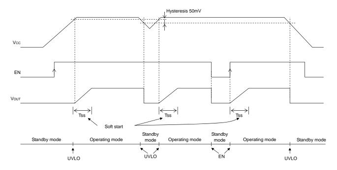
Fig.24 Soft start, Shutdown, UVLO timing chart
