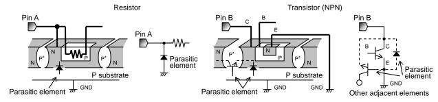
Fig.37 Simplified structure of monorisic IC
