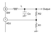
Fig.33 Determination of output voltage
