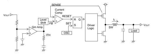
Fig.21 Diagram of current mode PWM control
