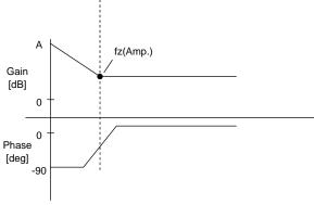
Fig.31 Error amp phase compensation characteristics
