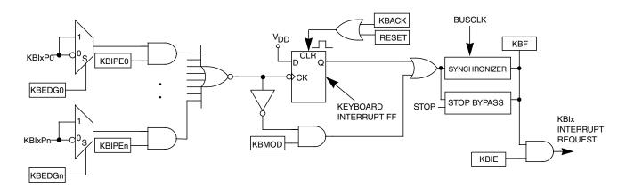
Figure 11-1. KBI block diagram
