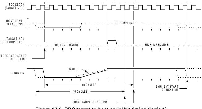
Figure 17-3. BDC target-to-host serial bit timing (logic 1)
