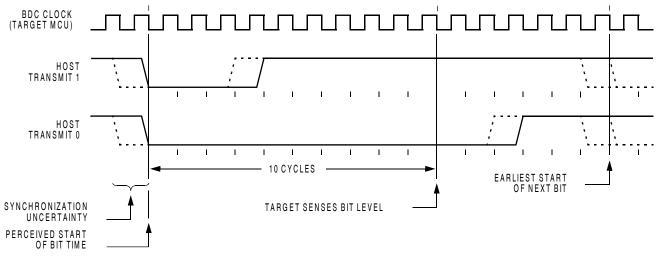
Figure 17-2. BDC host-to-target serial bit timing
