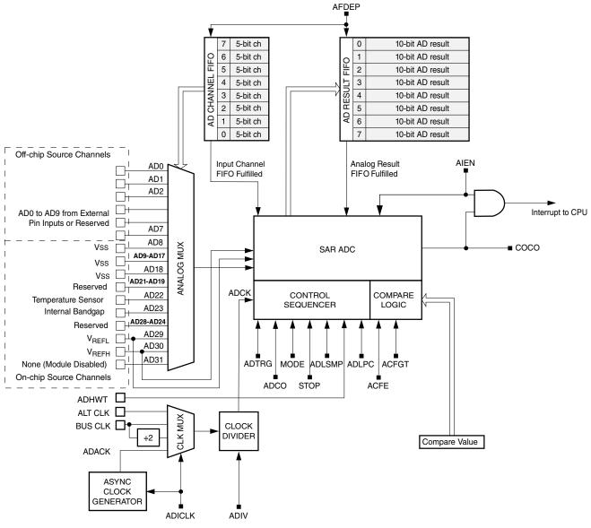
Figure 15-1. ADC Block Diagram
