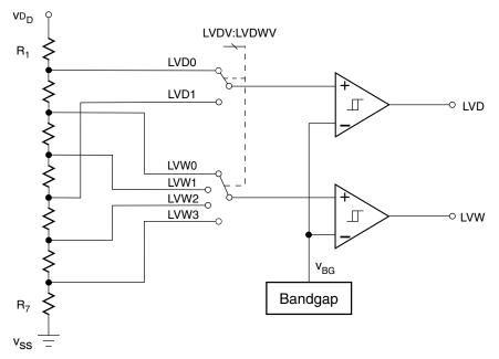
Figure 3-1. Low voltage detect (LVD) block diagram
