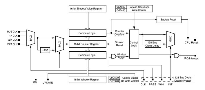
Figure 16-1. WDOG block diagram
