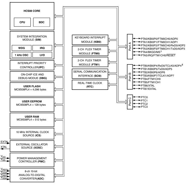
1. PTA4/BKGD/MS is an output-only pin when used as port pin. 2. PTB0 operates as true-open drain when working as output.
