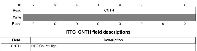
CNTH and CNTL contain the current value of the 16-bit counter. Writes have no effect to this register. Reset or writing different values to RTCLKS and RTCPS clear the count to 0x00.
