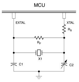
Figure 2-5. Typical crystal or resonator circuit
