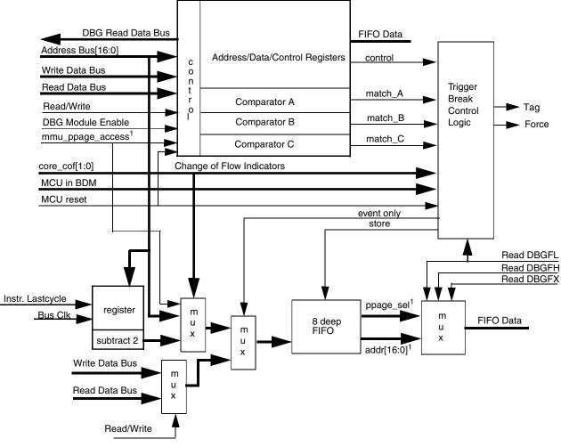
Figure 18-1. DBG block diagram
