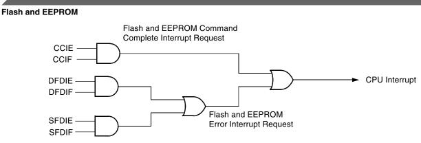
Figure 4-4. Flash and EEPROM module interrupts implementation
