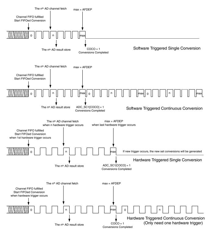
Figure 15-3. ADC FIFO conversion sequence
