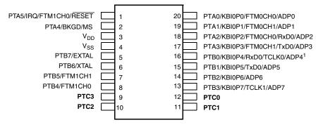
Pins in **bold** are not available on less pin-count packages. 1. True open drain pins
