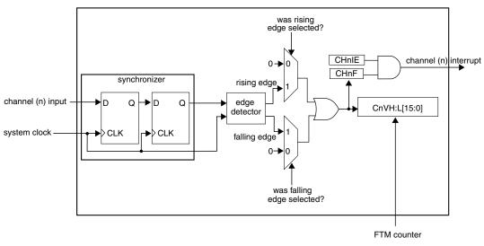
Figure 12-7. Input capture mode
