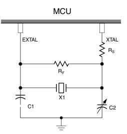
Figure 8-6. OSC high-gain mode connection
