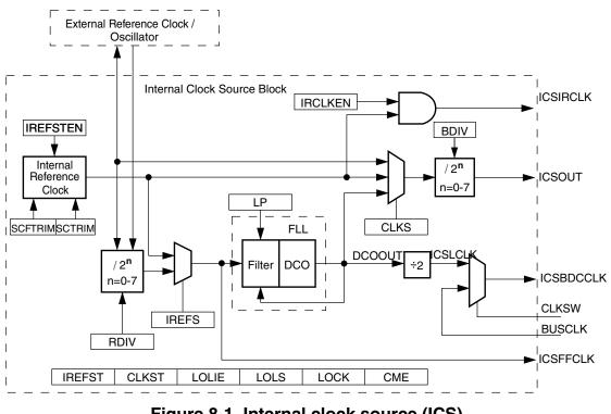
Figure 8-1. Internal clock source (ICS)
