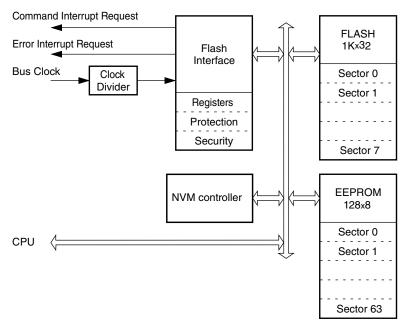
Figure 4-2. Flash and EEPROM block diagram
