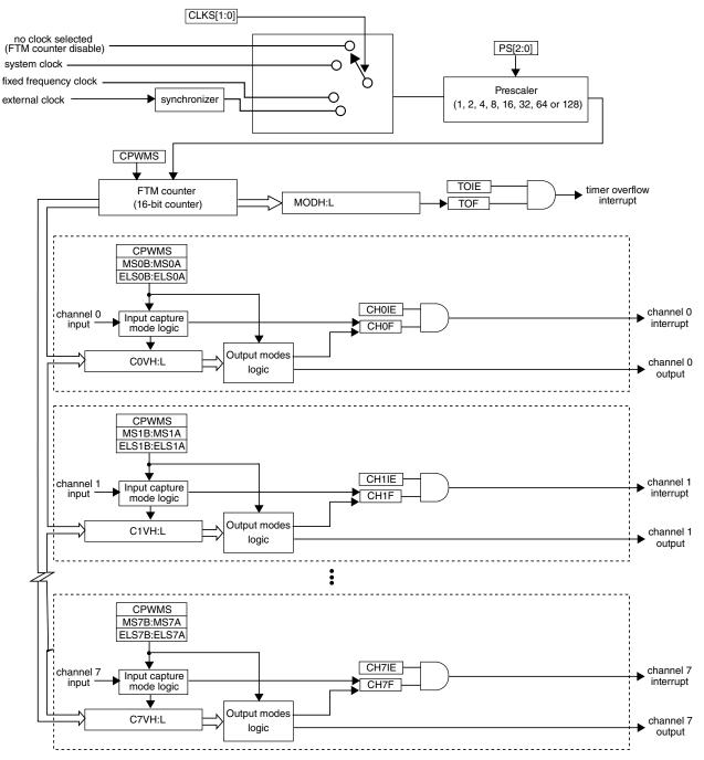
Figure 12-1. FTM block diagram
