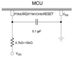
Figure 2-6. PTA5/IRQ/FTM1CH0/RESET external RC filter
