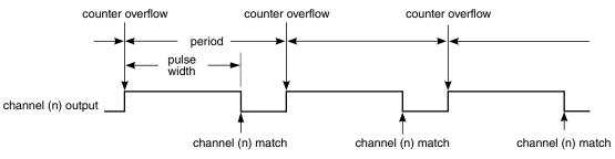
Figure 12-11. EPWM period and pulse width with ELSnB:ELSnA = 1:0
