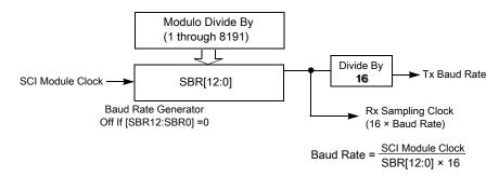
Figure 14-3. SCI baud rate generation
