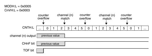
Figure 12-9. Example of the output compare mode when the match clears the channel output
