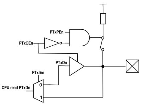
Figure 7-1. Normal I/O structure
