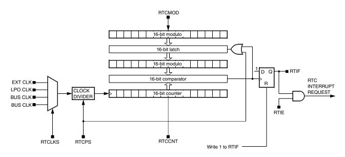
Figure 13-1. Real-time counter (RTC) block diagram
