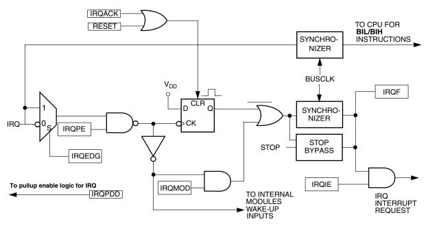
Figure 5-3. IRQ module block diagram
