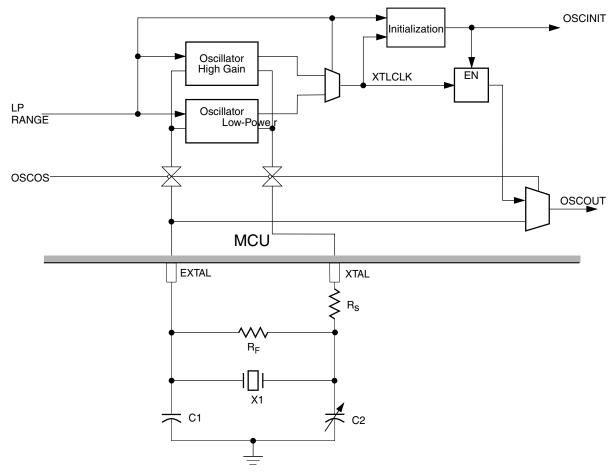
Figure 8-3. Oscillator module block diagram
