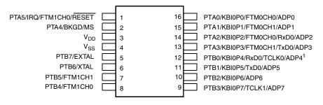
Pins in **bold** are not available on less pin-count packages. 1. True open drain pins
