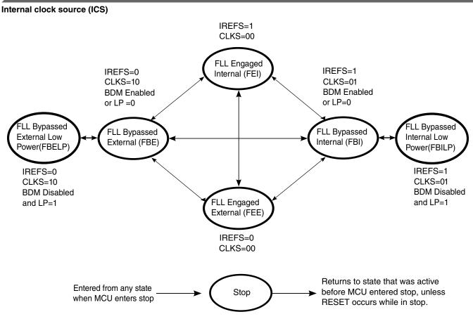
Figure 8-2. ICS clocking switching modes
