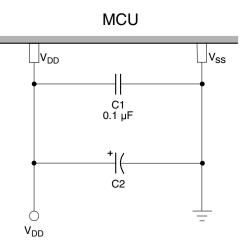
Figure 2-4. Power supply bypassing
