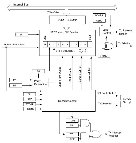
Figure 14-1. SCI transmitter block diagram
