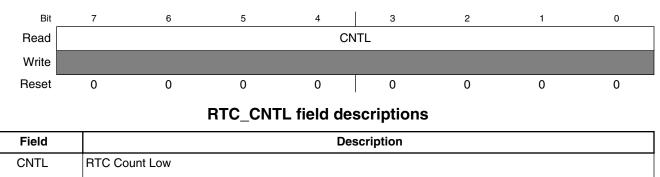
CNTH and CNTL contain the current value of the 16-bit counter. Writes have no effect to this register. Reset or writing different values to RTCLKS and RTCPS clear the count to 0x00.
