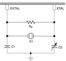
Figure 8-5. OSC low-power mode connection
