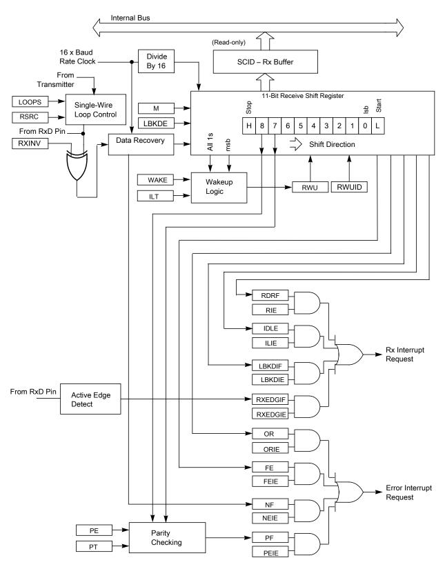
Figure 14-2. SCI receiver block diagram
