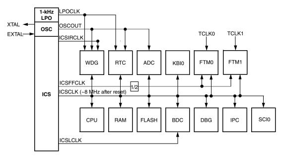
Figure 1-2. System clock distribution diagram
