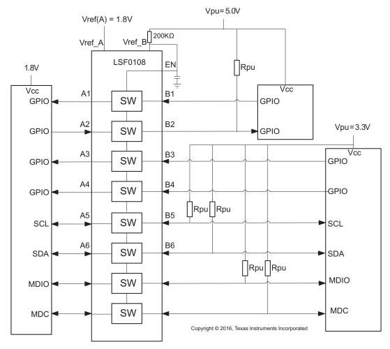
Figure 4. Bidirectional Translation to Multiple Voltage Levels
