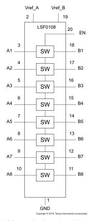
Figure 3. LSF0108-Q1 Functional Block Diagram
