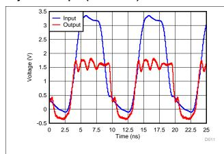
Figure 11. Waveform From TP1 (Pull-Up Resistor:  $160-\Omega$  and 50-pF Capacitance 3.3 V to 1.8 V at 100 MHz)
