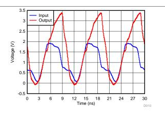
Figure 12. Waveform From TP2 (Pull-Up Resistor: 160- $\Omega$  and 50-pF Capacitance 1.8 V to 3.3 V at 100 MHz)
