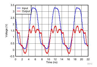
Figure 8. Translation Down (3.3 to 1.8 V) at 150 MHz
