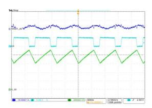
Figure 38. Output Ripple Voltage (V<sub>IN</sub>=5V, V<sub>OUT</sub>=3.3V, I<sub>OUT</sub>=800mA)
