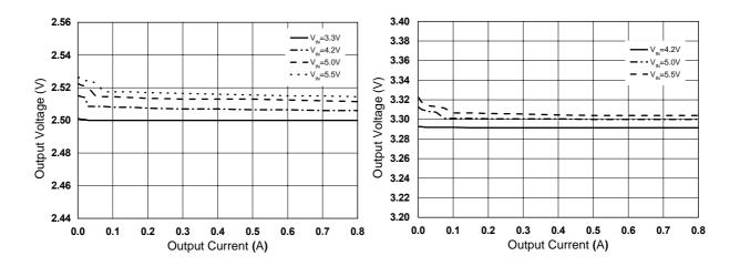
Figure 12. Load Regulation (V<sub>OUT</sub>=2.5±0.03V)
