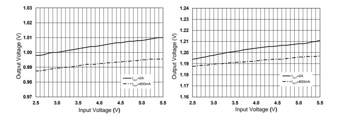
Figure 14. Line Regulation (V<sub>OUT</sub>=1.0±0.03V)
