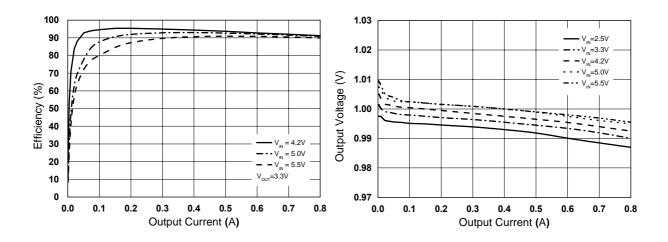
Figure 8. Efficiency vs. Output Current (V<sub>OUT</sub>=3.3V)
