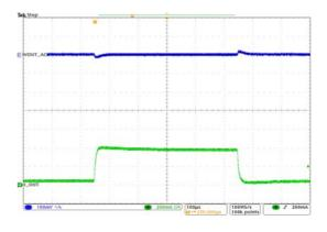
Figure 28. Short Circuit Recovery ( $V_{IN}$ =5.0V,  $V_{OUT}$ =3.3V,  $I_{OUT}$ =800mA)
