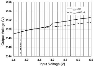
Figure 16. Line Regulation (V<sub>OUT</sub>=1.8±0.03V)
