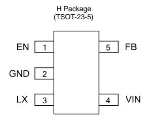
Figure 2. Pin Configuration of AUR9703 (Top View)
