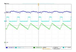
Figure 36. Output Ripple Voltage ( $V_{IN}$ =5V,  $V_{OUT}$ =3.3V,  $I_{OUT}$ =400mA)
