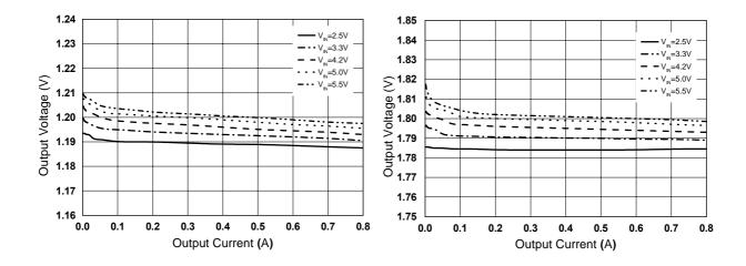
Figure 10. Load Regulation (V<sub>OUT</sub>=1.2±0.03V)
