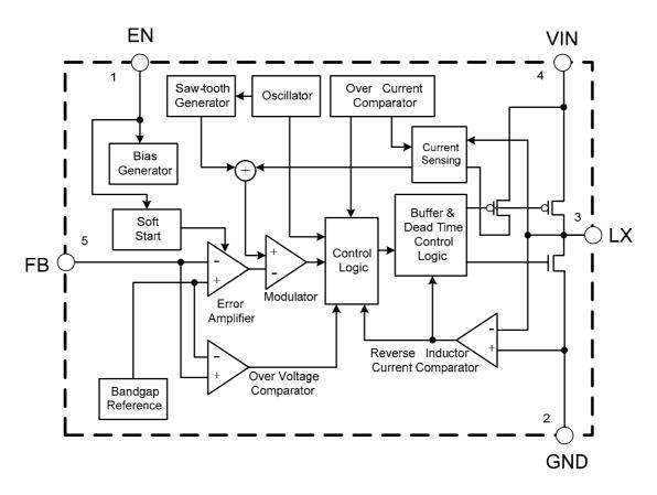
Figure 3. Functional Block Diagram of AUR9703
