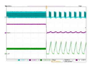
Figure 26. Shut Down through VIN (V<sub>IN</sub>=5.0 to 0V, V<sub>OUT</sub>=3.3V, I<sub>OUT</sub>=800mA)
