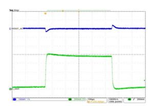
Figure 30. Load Transition (V<sub>IN</sub>=5.0V, V<sub>OUT</sub>=3.3V, I<sub>OUT</sub>=50mA to 400mA)
