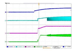
Figure 24. Shut Down through EN (V $_{\rm IN}=5V,~V_{\rm EN}=5V$  to 0V, V $_{\rm OUT}=3.3V,~I_{\rm OUT}=800mA)$
