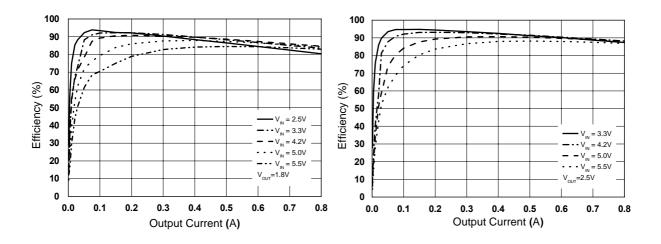
Figure 6. Efficiency vs. Output Current ( $V_{OUT}$ =1.8V)
