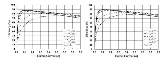
Figure 4. Efficiency vs. Output Current (V<sub>OUT</sub>=1.0V)
