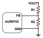
Figure 39. Setting the Output Voltage
