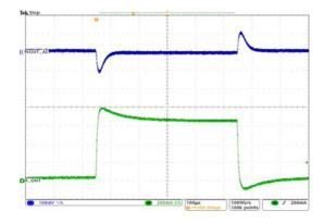
Figure 32. Load Transition ( $V_{IN}$ =5.0V,  $V_{OUT}$ =3.3V,  $I_{OUT}$ =50mA to 800mA)
