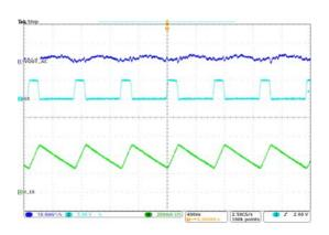
Figure 35. Output Ripple Voltage (V<sub>IN</sub>=5V, V<sub>OUT</sub>=1.0V, I<sub>OUT</sub>=400mA)
