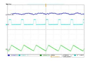
Figure 33. Output Ripple Voltage (V<sub>IN</sub>=5.0V, V<sub>OUT</sub>=1.0V, I<sub>OUT</sub>=10mA)
