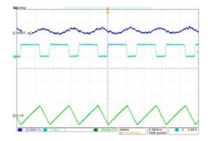
Figure 34. Output Ripple Voltage (V<sub>IN</sub>=5V, V<sub>OUT</sub>=3.3V, I<sub>OUT</sub>=10mA)
